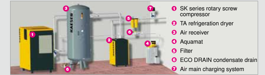
Compressed air supply system with separate components
